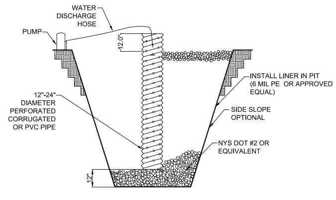
CONSTRUCTION SPECIFICATIONS SUMP PIT TO BE USED IN COORDINATION WITH ANTI-TRACKING/DECONTAMINATION PAD.
