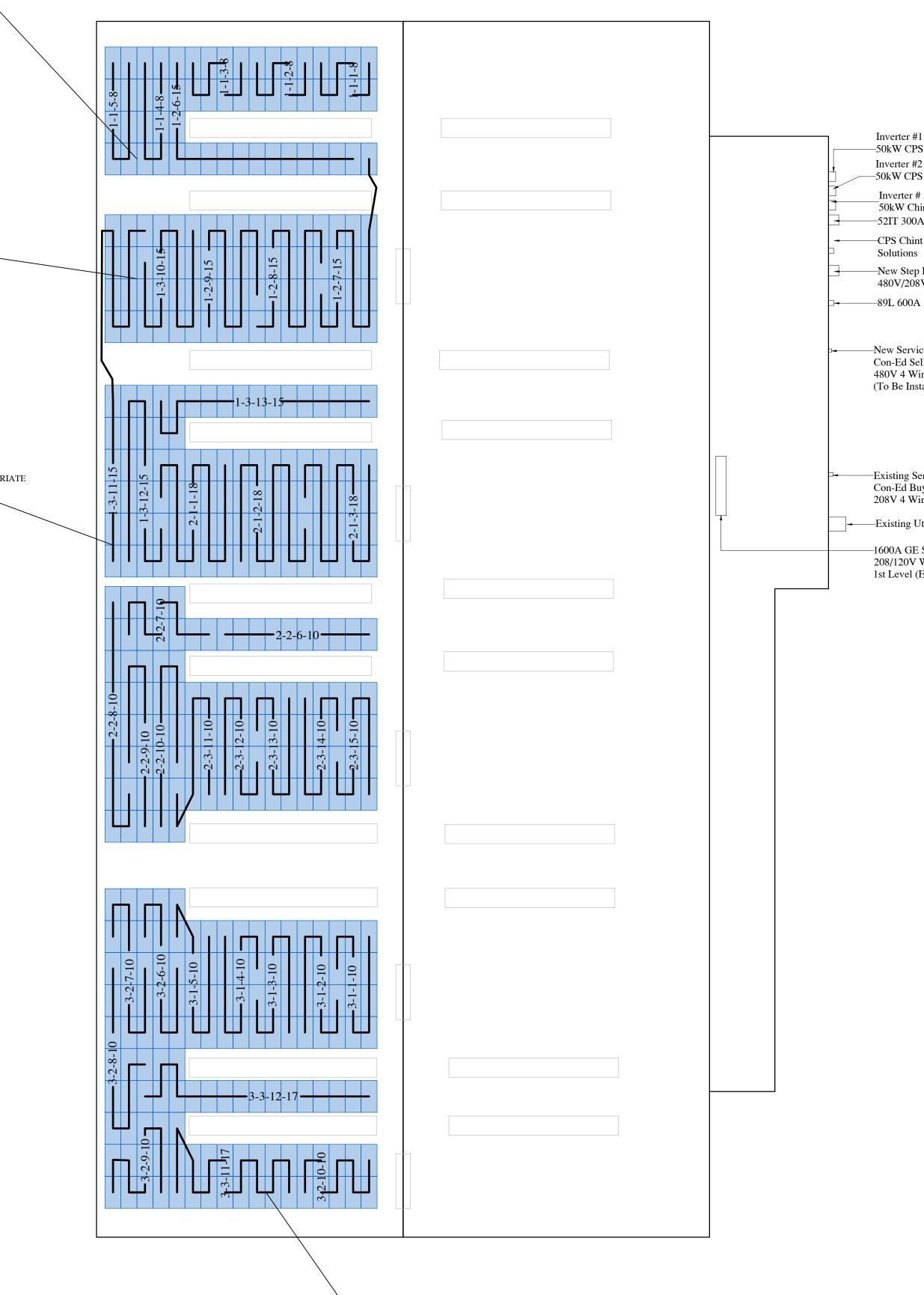
\DC WIRES TO BE SECURED BEHIND PANELS USING WEATHER APPROVED CABLE CLIPS IN AN ORGANIZED MANOR (SEE 1/E-003 FOR ADDITIONAL DETAILS)
